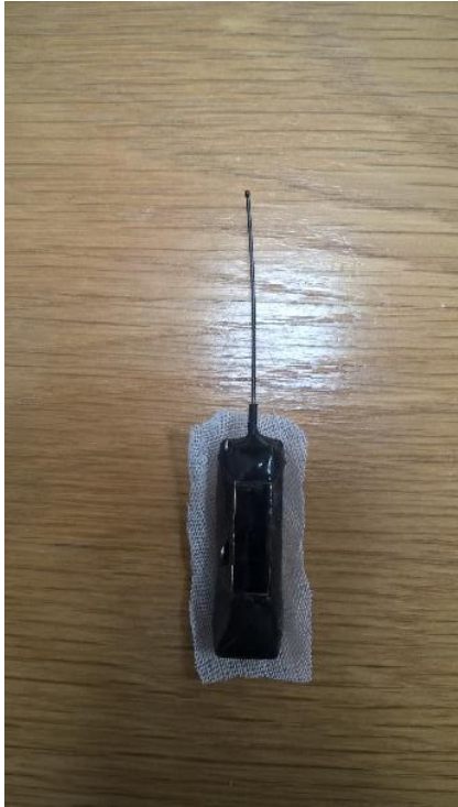
GPS/UHF tags with small solar panel
