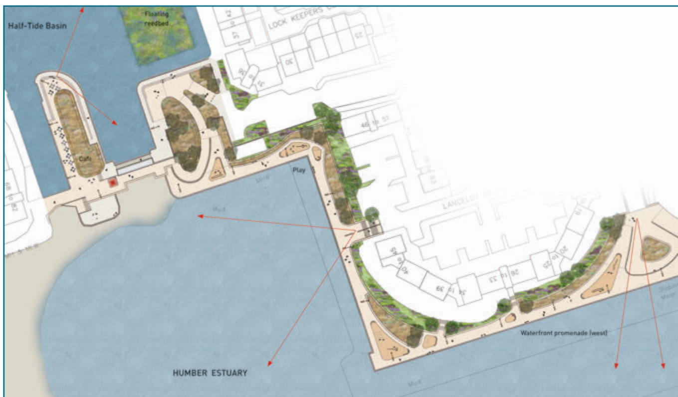
Exemplar opportunities to improve green infrastructure alongside flood defence improvements at Hull - Environment Agency/Sheils Flynn
